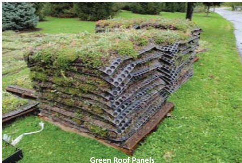
Green Roof Panels
